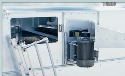
External Motor Mount (Optional Ladder Shown)
